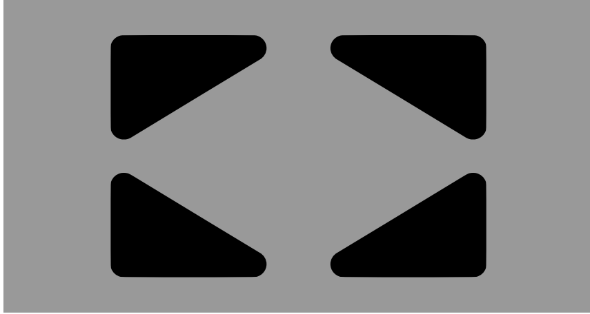
Figure 3: It is recommended to precut cooktop cut outs as shown here, then finish the cut on site. This will provide enough strength during transportation to avoid breakage.
